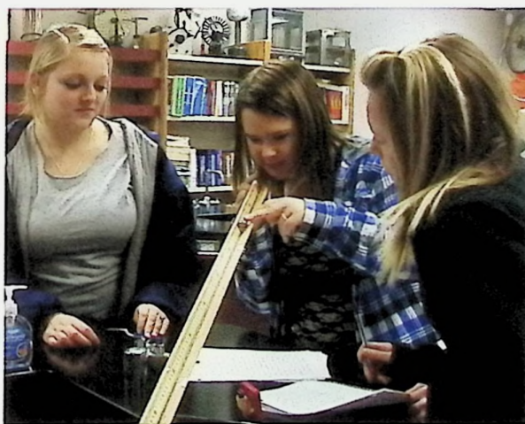
Katie Fuller releases the marble down a path between the meter stick ramp while group members Mariah Spriggs and Faith Francis closely observe and take notes. The Physics students stopped and started the marble at specific time intervals in order to later create a position-time graph.
